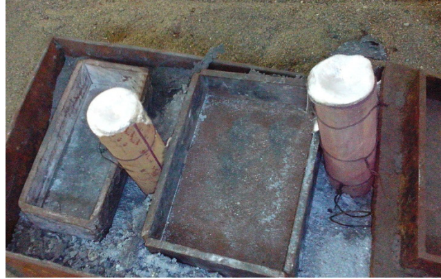
Fig: Mould and cast product after casting
